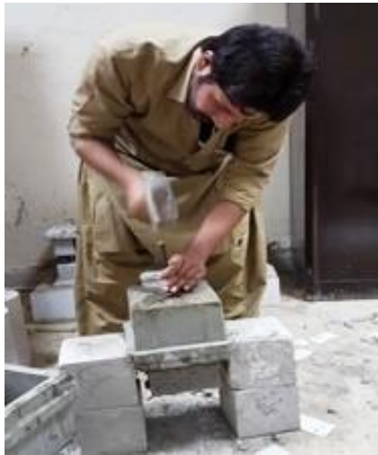
Figure. 5: Demoulding of cubes specimen
