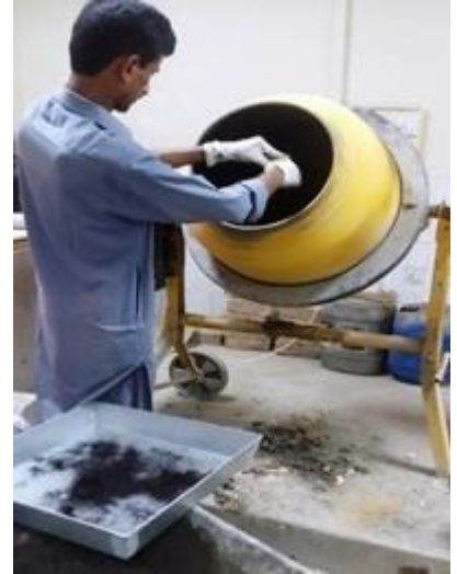
Figure. 3: Addition of Hair Fiber in concrete mix
