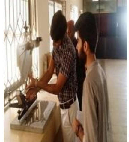
Figure. 9: Skid resistance test of slab specimen
