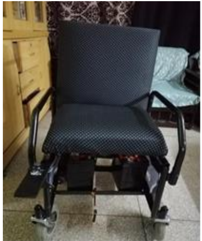
Fig. 5. Complete Final Wheelchair with all features.
