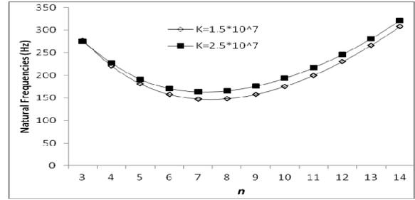
**Fig. 4 Comparison of the variation of natural frequencies (Hz) of submerged isotropic cylindrical shells against circumferential wave number  $n$ , for different values of Winkler foundation for simply supported-simply supported end condition ( $m=1$ ,  $L=0.41$ ,  $R=0.3015$ ,  $h=0.001$ ,  $E=2.1 \times 10^{11} \text{ N/m}^2$ ,  $\nu=0.3$ ,  $\rho = 7850 \text{ kg/m}^3$ ,  $G=0$ )**
