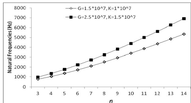
**Fig. 8 Comparison of the variation of natural frequencies (Hz) of submerged isotropic cylindrical shells against circumferential wave number  $n$ , for different values of Pasternak and Winkler foundations for simply supported-simply supported end condition ( $m=1, L=0.41, R=0.3015, h=0.001, E=2.1 \times 10^{11} \text{ N/m}^2, \nu=0.3, \rho=7850 \text{ kg/m}^3$ )**
