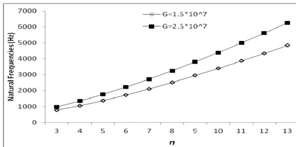
**Fig. 6 Comparison of the variation of natural frequencies (Hz) of submerged isotropic cylindrical shells against circumferential wave number  $n$ , for different values of Pasternak foundation for simply supported-simply supported end condition ( $m=1, L=0.41, R=0.3015, h=0.001, E=2.1 \times 10^{11} \text{ N/m}^2, \nu=0.3, \rho=7850 \text{ kg/m}^3, K=0$ )**
