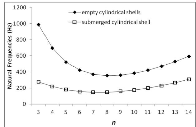
**Fig. 2** Comparison of the variation of natural frequencies (Hz) of empty and submerge isotropic cylindrical shells against circumferential wave number  $n$ , for simply supported-simply supported end condition having shell parameters ( $m=1, L=0.41, R=0.3015, h=0.001, E=2.1 \times 10^{11} N/m^2, \nu=0.3, \rho =7850kg/m^3, G=0, K=1.5 \times 10^7$ )
