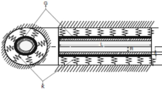
Fig. 1 Cylindrical shell on elastic foundation
