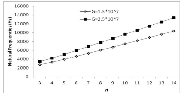
**Fig. 5 Comparison of the variation of natural frequencies (Hz) of empty isotropic cylindrical shells against circumferential wave number  $n$ , for different values of Pasternak foundation for simply supported-simply supported end condition ( $m=1$ ,  $L=0.41$ ,  $R=0.3015$ ,  $h=0.001$ ,  $E=2.1 \times 10^{11} \text{ N/m}^2$ ,  $\nu=0.3$ ,  $\rho = 7850 \text{ kg/m}^3$ ,  $K=0$ )**
