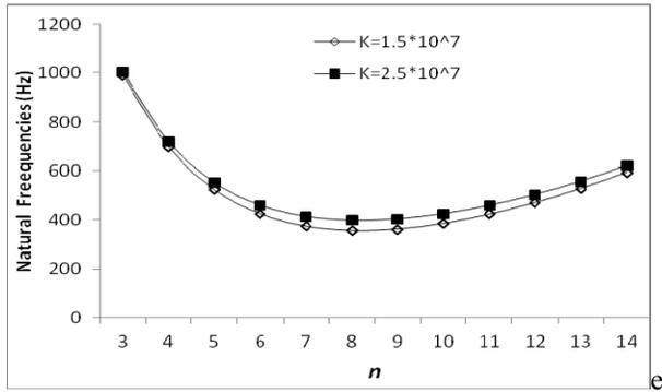
**Fig. 3 Comparison of the variation of natural frequencies (Hz) of empty isotropic cylindrical shells against circumferential wave number  $n$ , for different values of Winkler foundation for simply supported-simply supported end condition ( $m=1$ ,  $L=0.41$ ,  $R=0.3015$ ,  $h=0.001$ ,  $E=2.1 \times 10^{11} \text{ N/m}^2$ ,  $\nu=0.3$ ,  $\rho = 7850 \text{ kg/m}^3$ ,  $G=0$ )**
