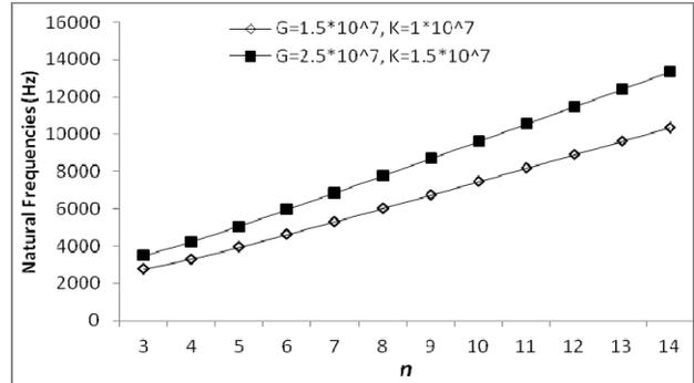
**Fig. 7 Comparison of the variation of natural frequencies (Hz) of empty isotropic cylindrical shells against circumferential wave number  $n$ , for different values of Pasternak and Winkler foundations for simply supported-simply supported end condition ( $m=1, L=0.41, R=0.3015, h=0.001, E=2.1 \times 10^{11} \text{ N/m}^2, \nu=0.3, \rho=7850 \text{ kg/m}^3$ )**
