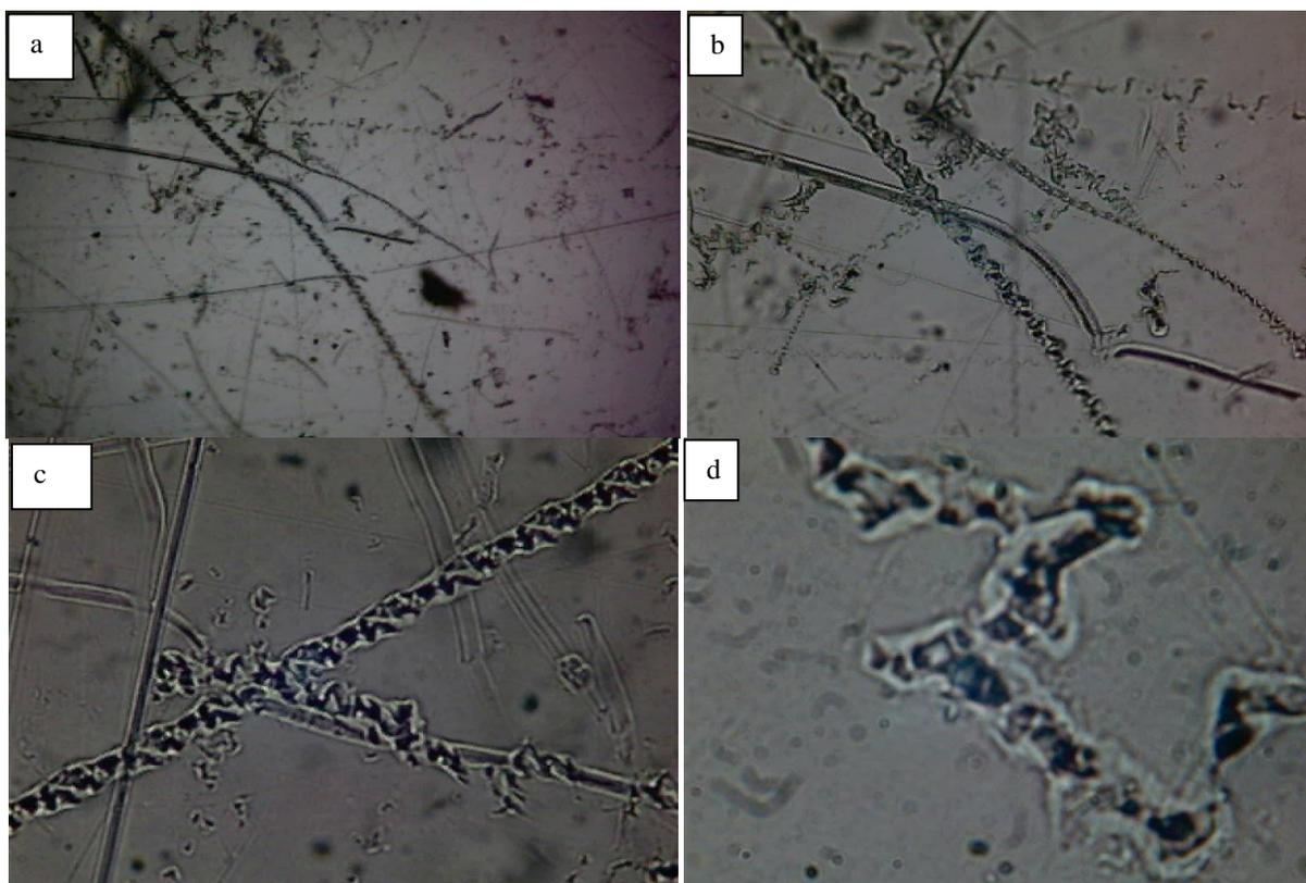
**Fig- 6: Micrographs of PVC irradiated by laser produced lead ions at 300 V show chain scission and linking at magnification. (a) 40, (b) 100, (c) 100 (d) 1000.**
