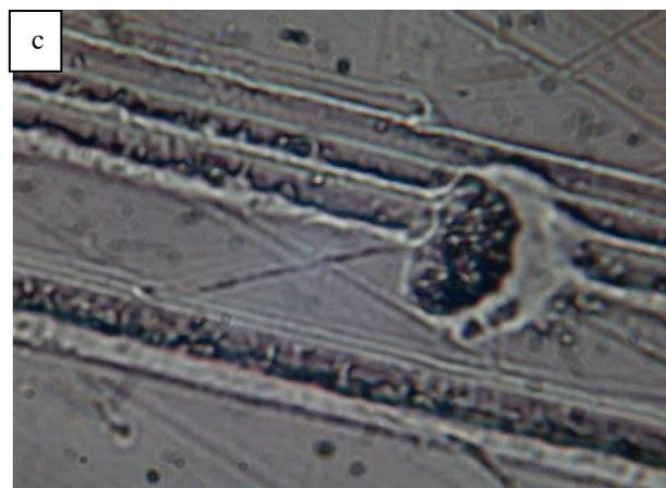
**Fig- 4: Micrographs of PVC irradiated by laser produced lead ions at 100 V show craters and cracking, at magnification of (a) 100, (b) 400 and (c) 100.**
