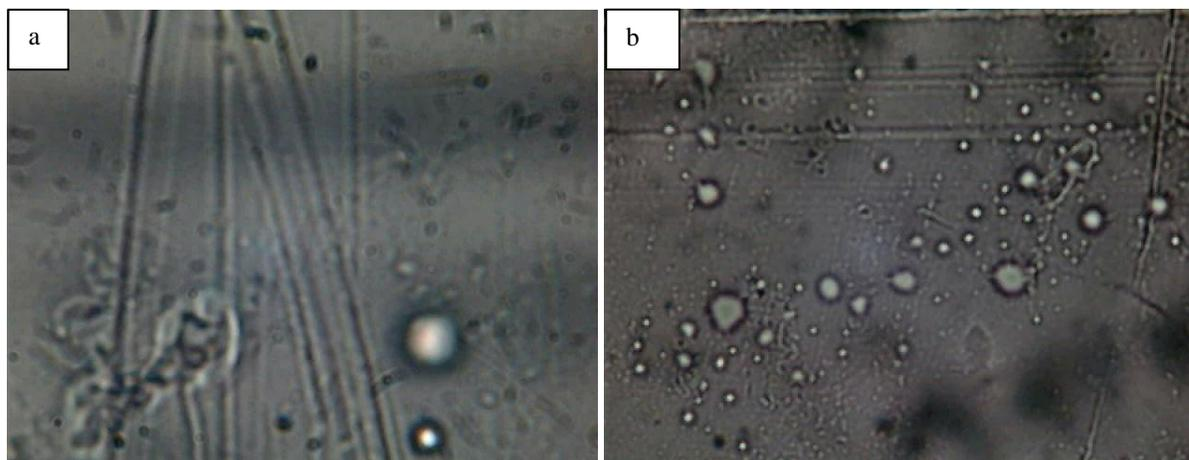
Fig- 7: Micrographs of PVC irradiated by laser produced lead ions at 300 V showing surface burning at magnification, (a) 400, (b) 1000.
