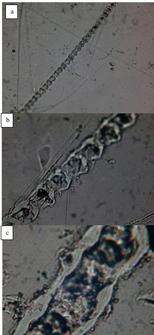
**Fig-2: Micrographs of PVC irradiated by laser lead at 0 V showed Chain scission at magnification of (a) 100, (b) 400 and (c) 1000.**
