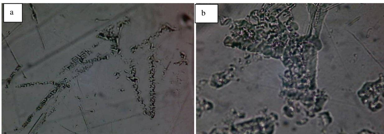
Fig- 8: Micrographs of PVC irradiated by laser produced lead ions at 300 V show cluster formation at magnification of (a) 100 and (b) 400.
