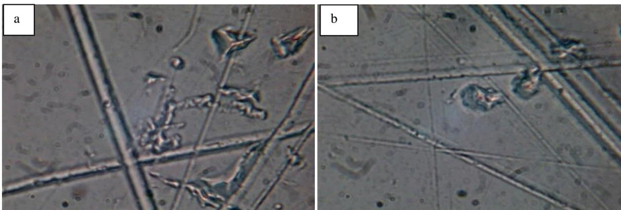
**Fig- 5: Micrographs of PVC irradiated by laser produced lead ions at 100 V show thermal sputtering (a & b) at magnification 1000.**
