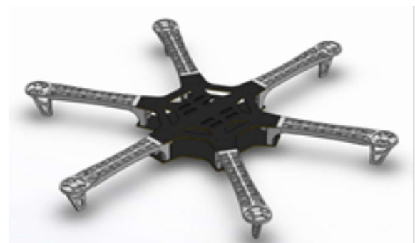
Figure 6. 3D model of hexagonal structure of design 2
