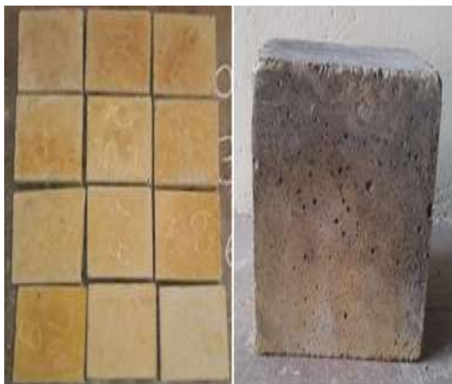
Fig. 4. Concrete exposed to 1% Hydrochloric Acid.
