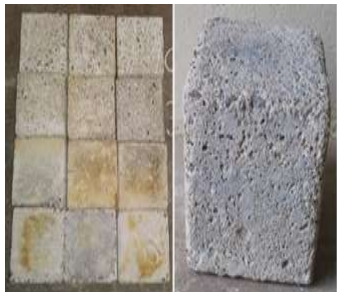
Fig. 6. Concrete exposed to 1% Sulphuric Acid.
