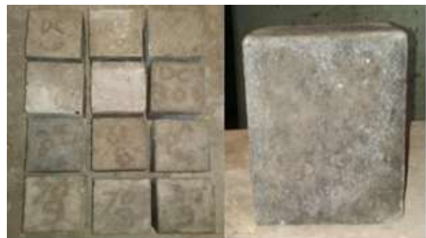
Fig. 7. Concrete exposed to Marine water.
