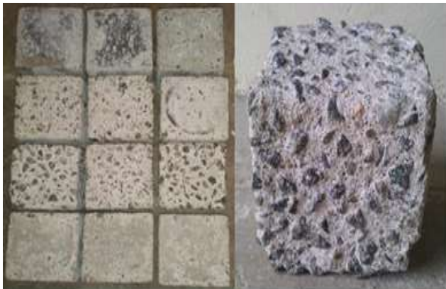
Fig. 7. Concrete exposed to 5% Ammonium sulphate solution.
