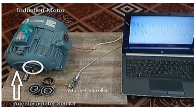
Figure 1: Complete working setup.
