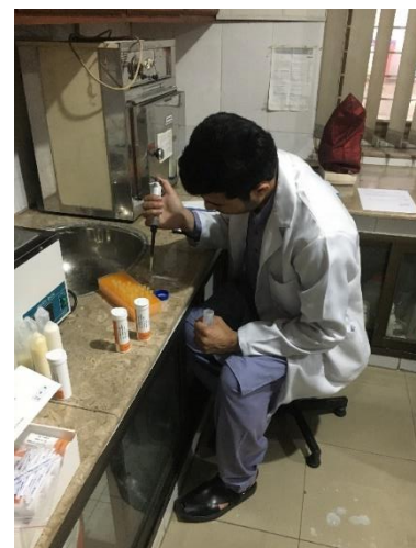
Figure 1: Microwells and dipsticks Figure 2: Taking 200µl milk sample Figure 3: Pouring 200µl milk sample in microwell before inserting the dipstick.
