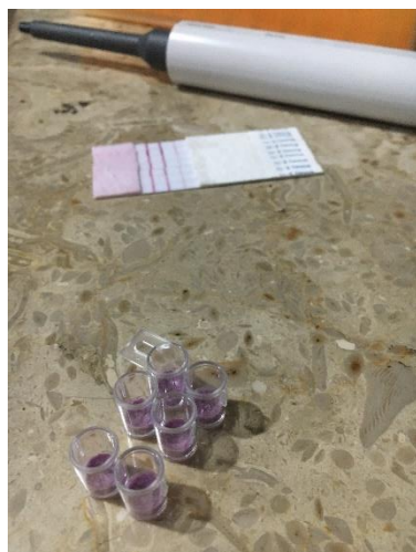
Figure 1: Microwells and dipsticks Figure 2: Taking 200µl milk sample Figure 3: Pouring 200µl milk sample in microwell before inserting the dipstick.
