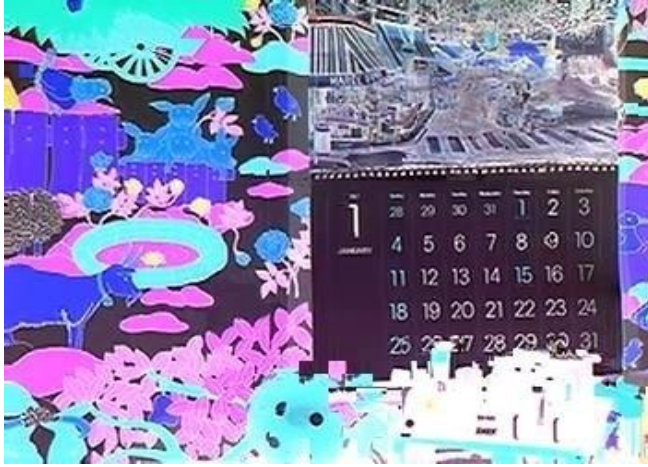
AVC encoded video with SE at QP 24 for Mobile with CABAC [Y=6.7, U=12.9, V=13.3] dB, SSIM =0.0698.
