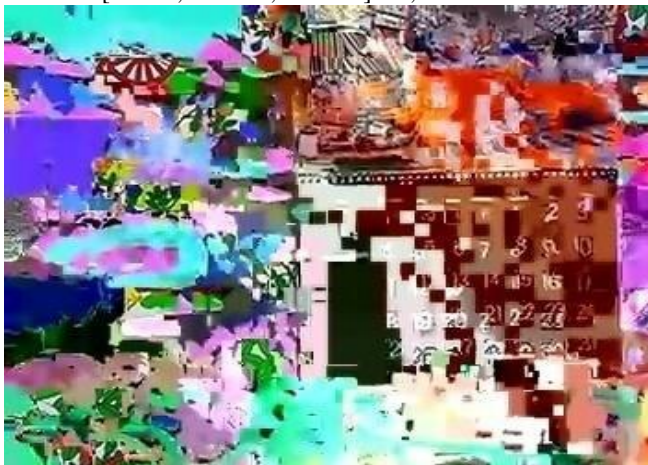
AVC encoded video with SE at QP 48 for Mobile with CABAC [Y=7.6, U=14.4, V=13.2] dB, SSIM =0.0690.
