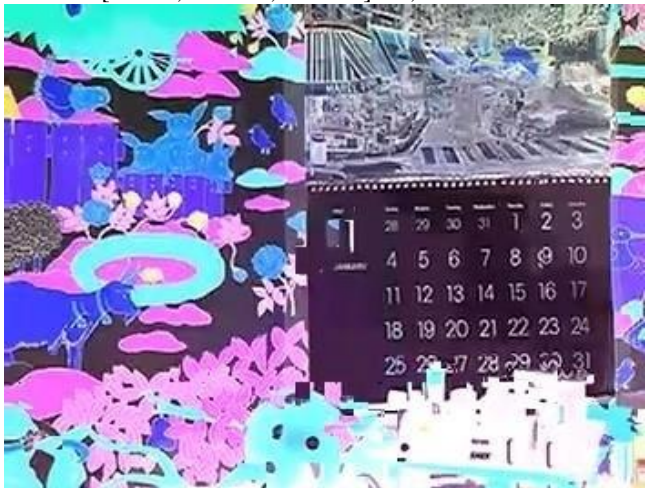
AVC encoded video with SE at QP 36 for Mobile with CABAC [Y=6.6, U=12.9, V=13.4] dB, SSIM =0.0805.
