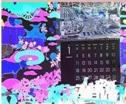
AVC encoded video with SE at QP 12 for Mobile with CABAC [Y=6.7, U=12.9, V=13.2] dB, SSIM =0.0637.
