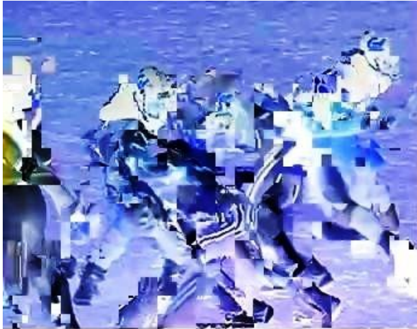
AVC encoded video with SE at QP 36 for Football with CABAC [Y=9.6, U=14.1, V=21.2] dB, SSIM =0.6304.
