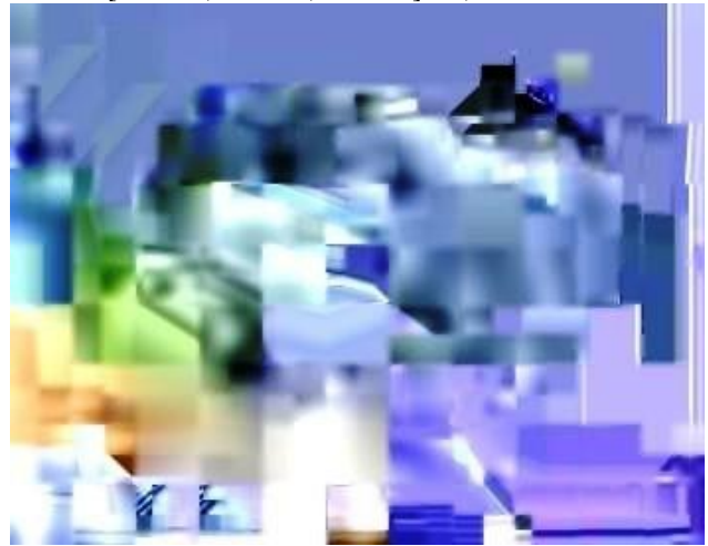
HEVC encoded video with SE at QP 48 for Football with CABAC [Y=9.6, U=13.4, V=20.0] dB, SSIM =0.7063.
