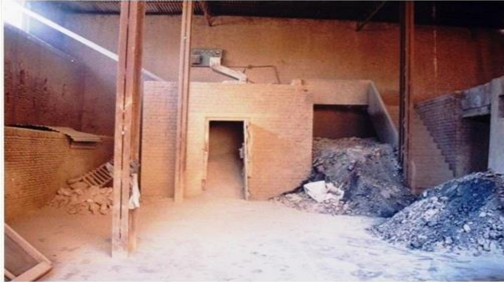
Figure 5: The granulated form of Kankar lime collected below the roof in cabin
