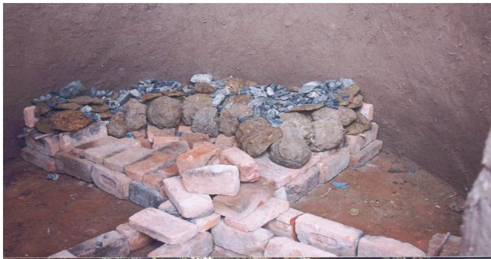
Figure 4: A layer of fuel (cow dung cakes and coal) before loading the Kankar lime
