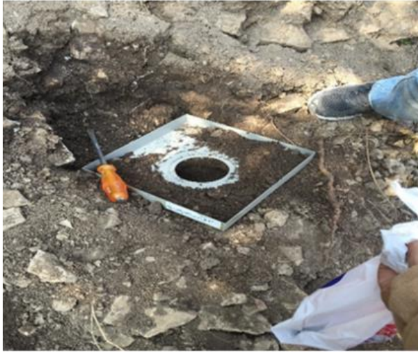
Fig- 2: In-situ density determination by sand replacement method along the failure surface.
