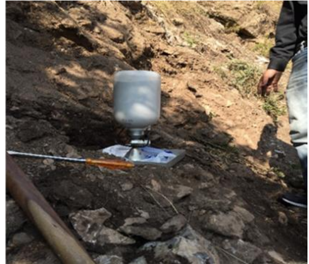
Fig- 2: In-situ density determination by sand replacement method along the failure surface.
