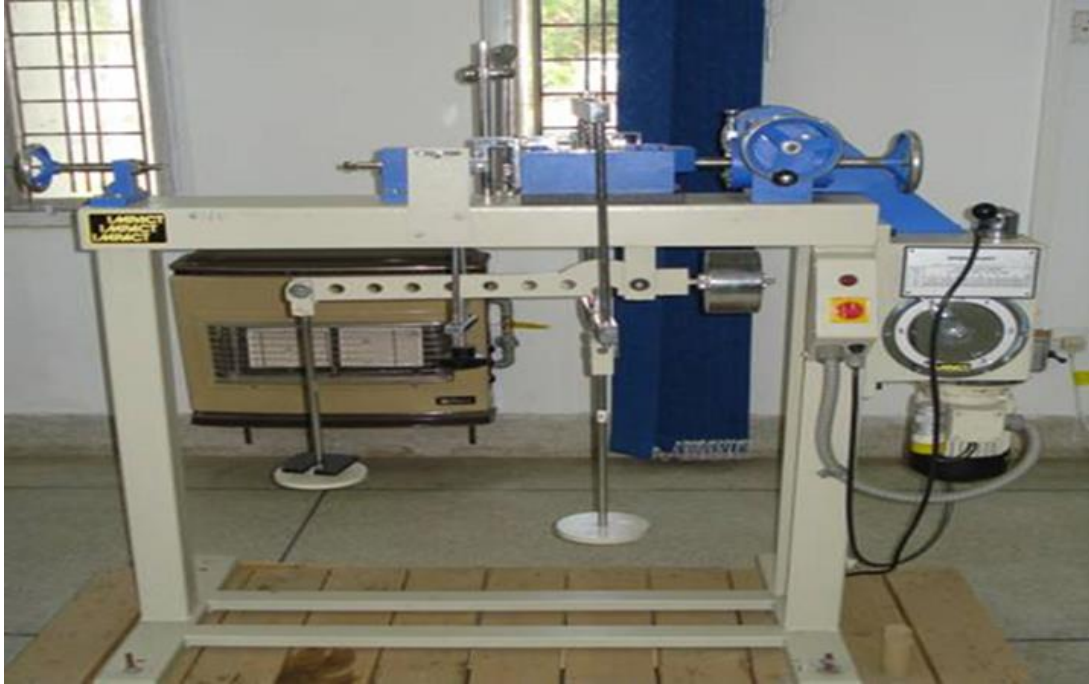
Fig- 3: Simple Direct shear test apparatus used for this study
