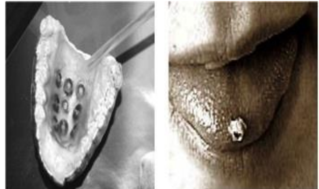
Figure 2. Left: The palatal plate (placed on a mould of the upper part of the mouth) with inductive coils and a silicone tube leading the wires out of the mouth. Right: The activation unit glued to the tongue.
