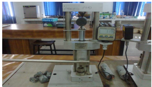
Figure 2 – Determination of point load index of dolerite
