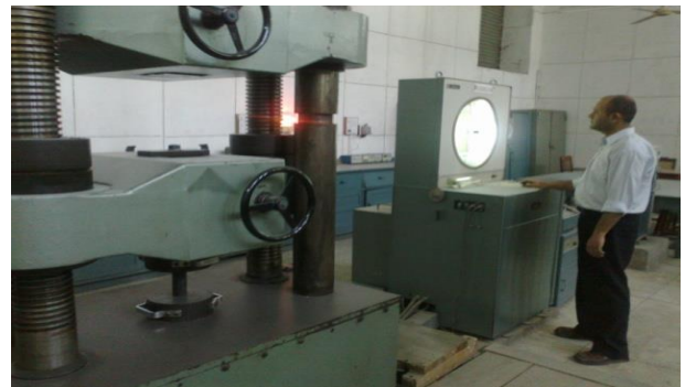
Figure 1 – Determination of uniaxial compressive strength of dolerite by direct testing method
