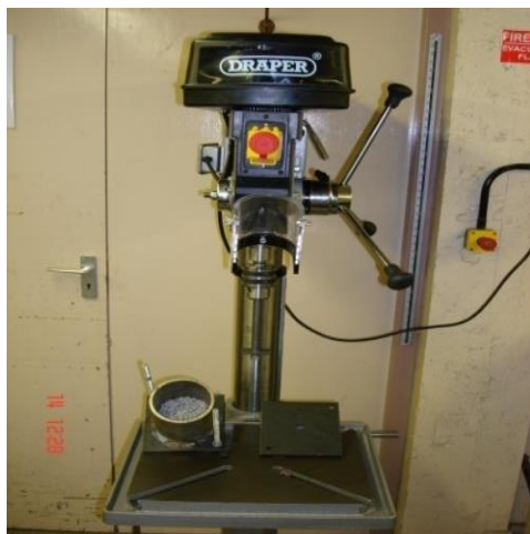
Figure 1. Pillar drill machine at the University of Leeds, UK used for LCPC test.
