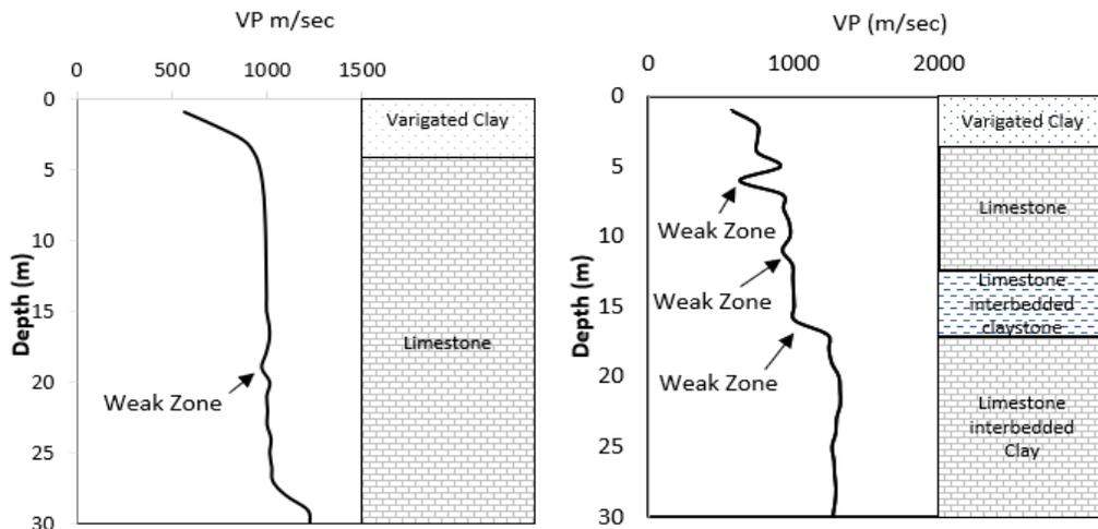
Figure-2. The Downhole seismic record a) The profile of  $V_p$  recorded in BH-1 b) The profile of  $V_p$  record in BH-2. The lithology column is placed
