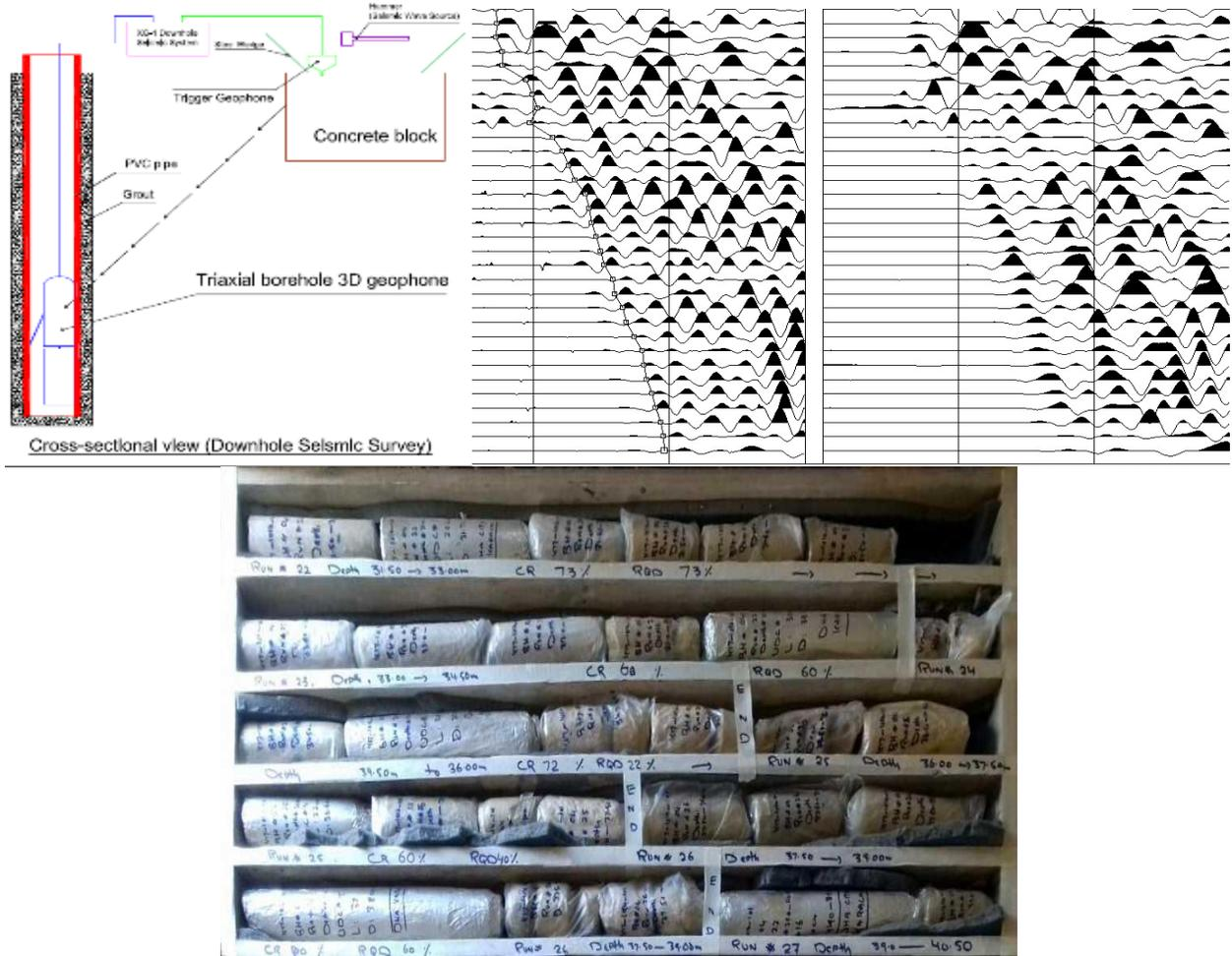
Figure-1. A) Schematic diagram of downhole seismic acquisition B) Seismic wave picking from BH-1 c) Seismic wave picking from BH-2 D) Core samples from specific depth in boreholes.
