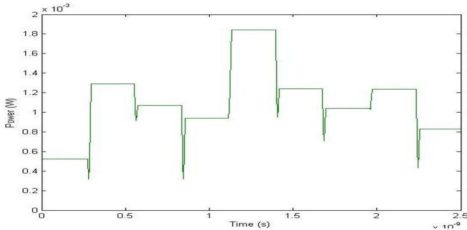
**Figure-7: Optical Signal in time domain before the signal enters the fiber**
