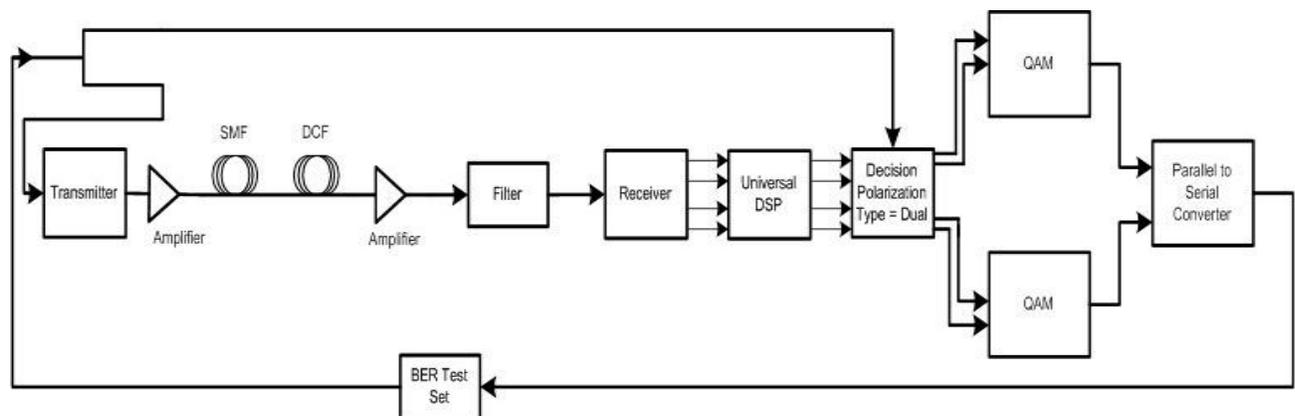
Figure-1: Block diagram of 112-Gbit/s Dual Polarization 128-QAM Communication Model
