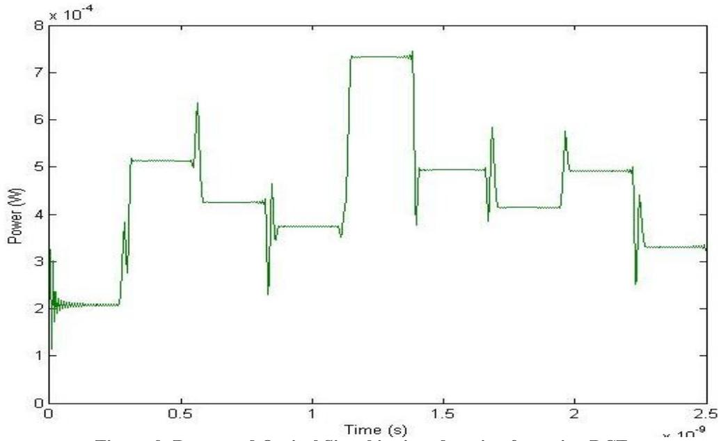
**Figure-9: Recovered Optical Signal in time domain after using DCF**
