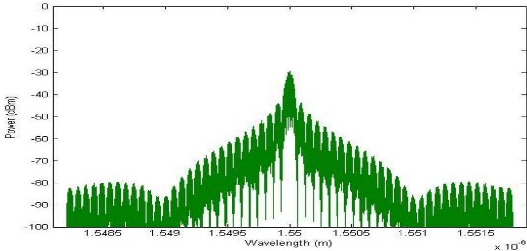
**Figure-4: Optical Spectrum before the signal enters the fiber**
