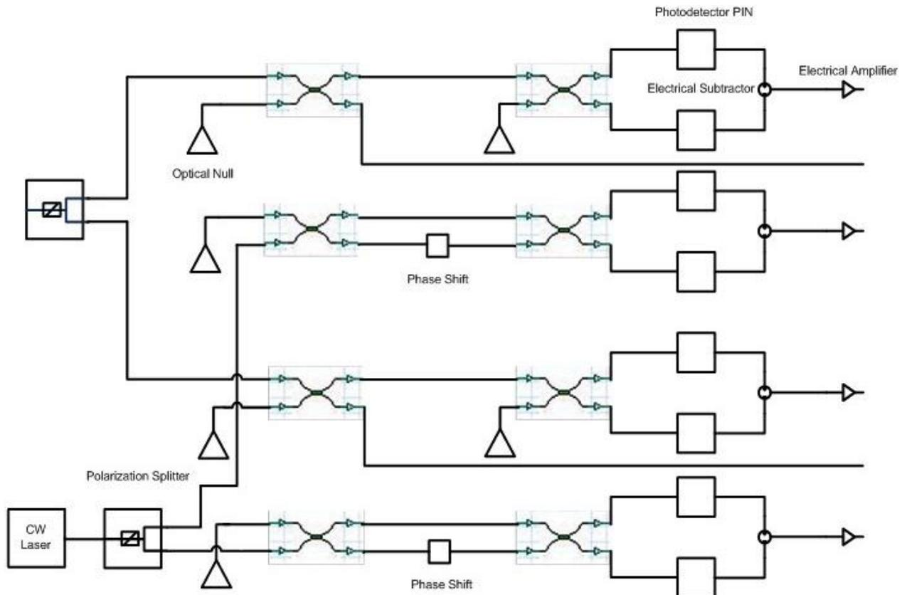
**Figure-3: Schematic diagram of 128-QAM Receiver**
