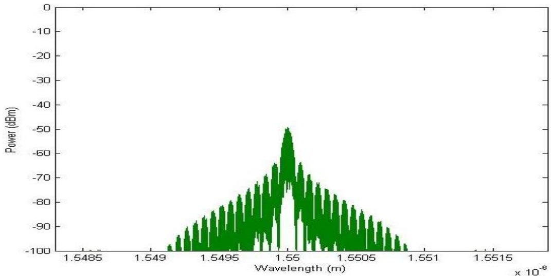
**Figure-5: Optical Spectrum after the signal passes through the fiber**
