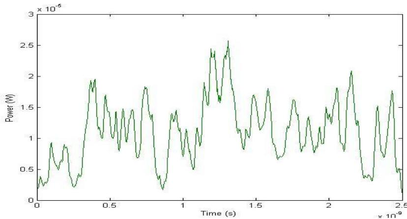
**Figure-8: Distorted Optical Signal in time domain after passing through the fiber**
