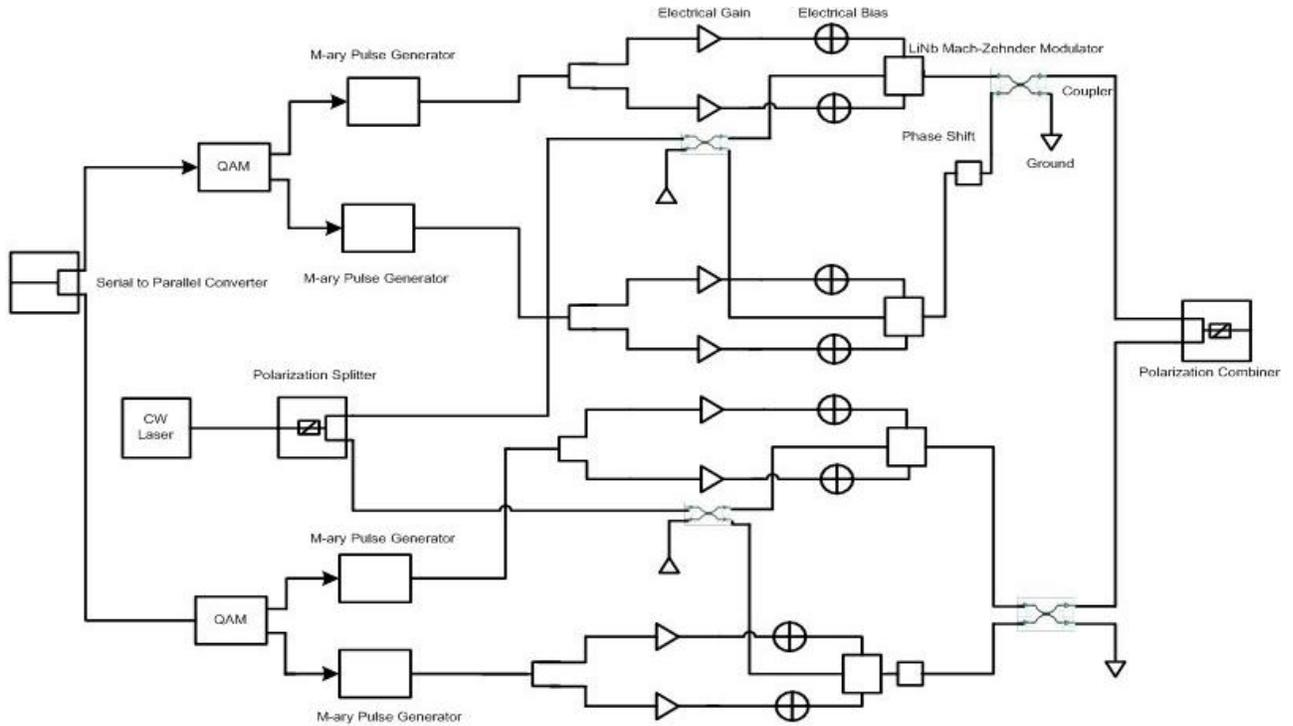
**Figure-2: Schematic diagram of 128-QAM Transmitter**
