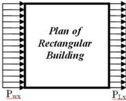
Figure 2: Full Design Wind Pressure Acting on Both Sides
