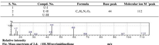
Fig. Mass spectrum of 2,4- (1H,3H)pyrimidinedione
