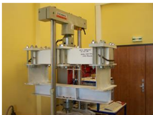
Fig. 2: Experimental setup for reverse cyclic bending test on beam
