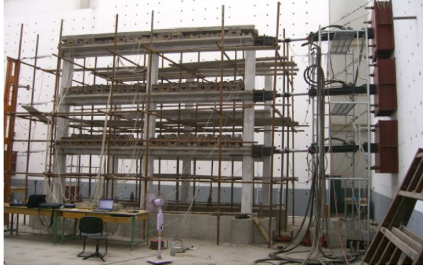
Figure 5. Experimental setup of tested frames
