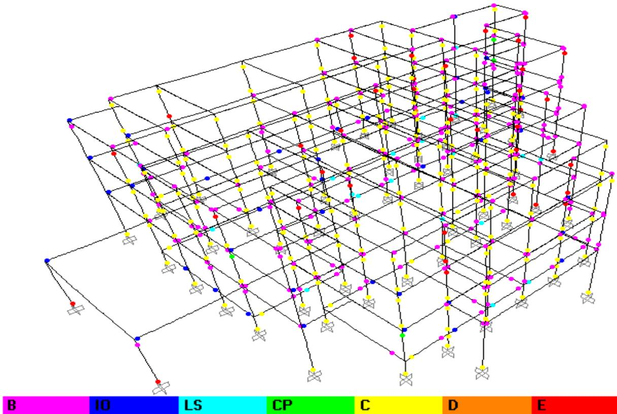
Figure – 5. Damage Degree at End of Analysis of Existing Building in X-Direction.
