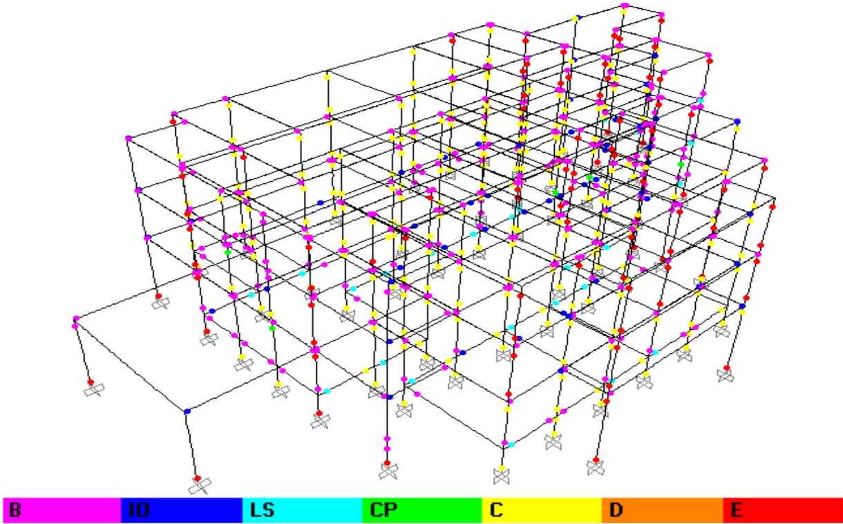
Figure – 4. Damage Degree at End of Analysis of Original Building in X-Direction
