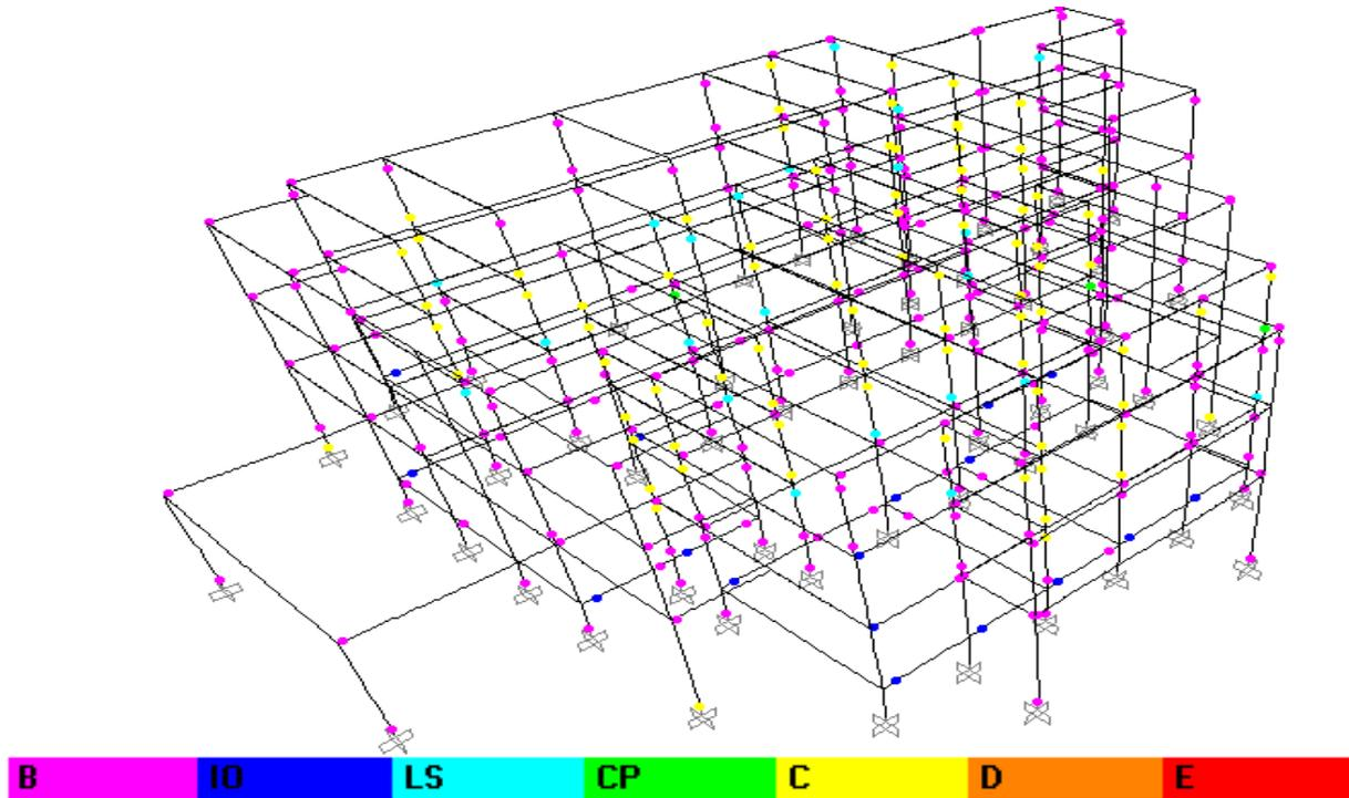
Figure – 8. Damage Degree of Retrofitted Building at a Displacement of 148mm in X-Direction
