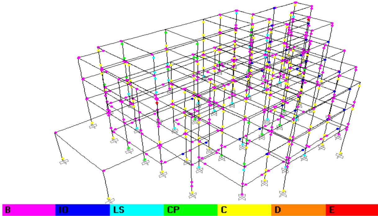
**Figure – 6. Damage Degree of Original Building at a Displacement of 148mm in X-Direction**
