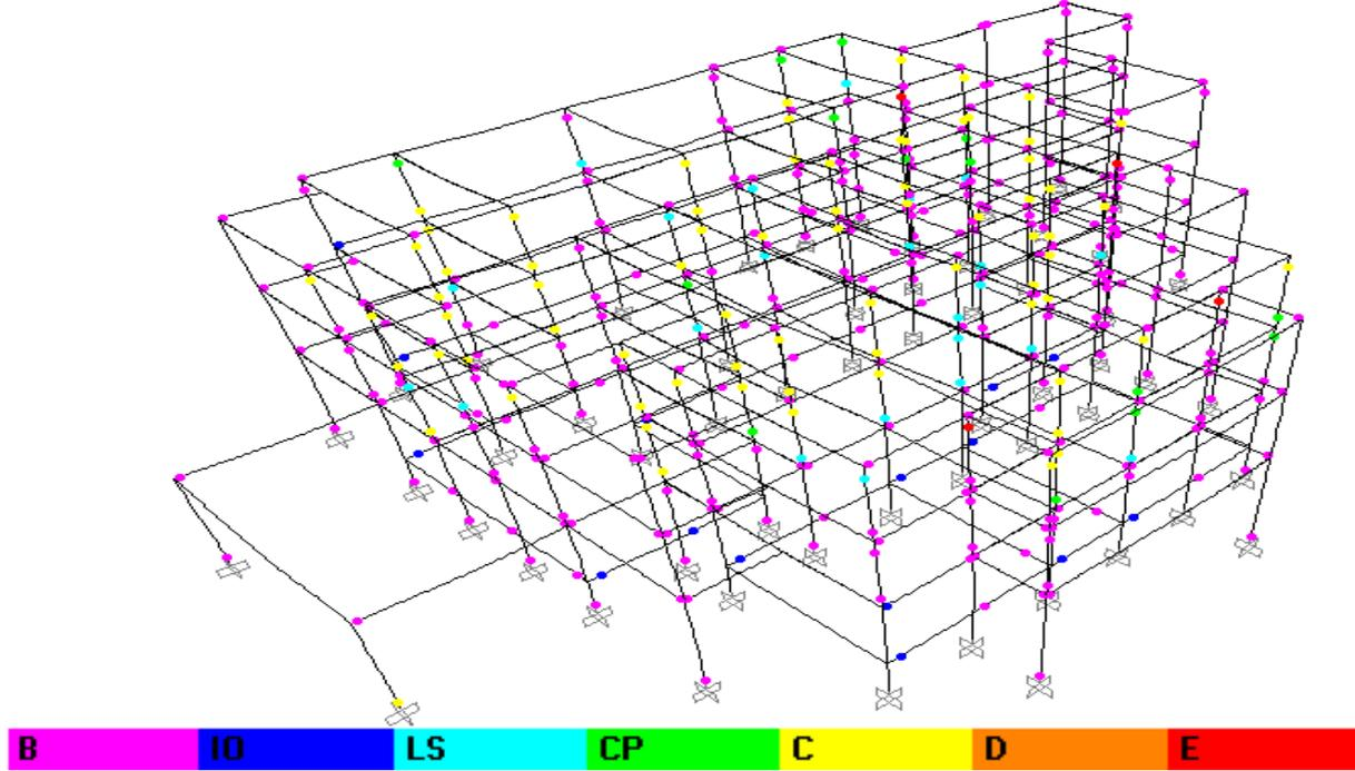
**Figure – 7. Damage Degree of Existing Building at a Displacement of 148mm in X-Direction**
