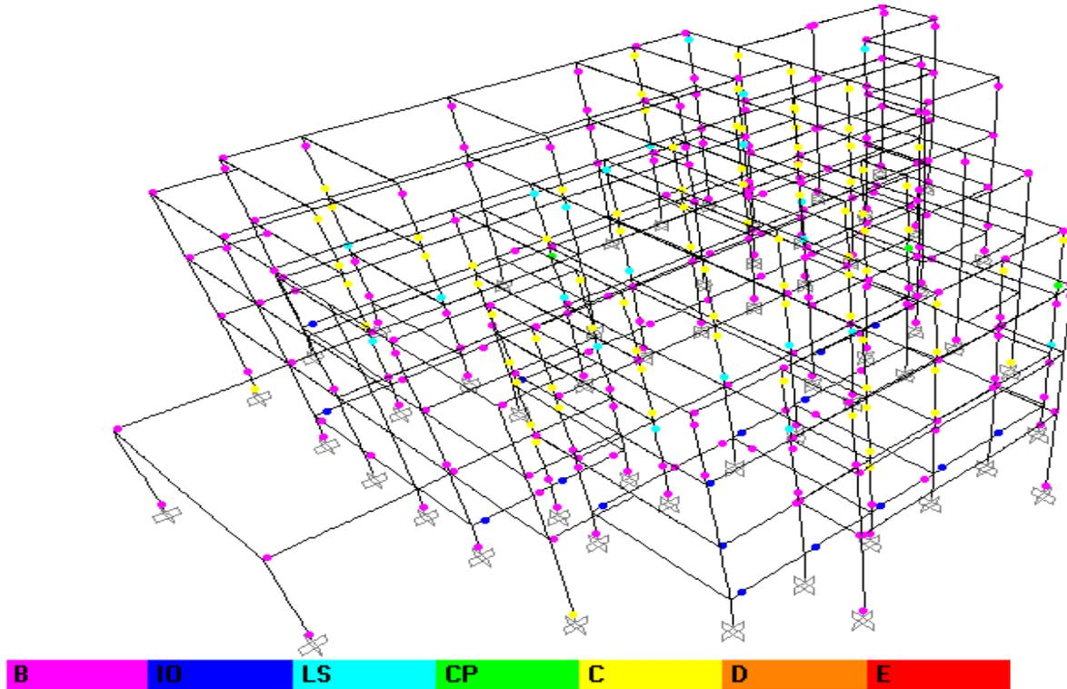
Figure -3. Damage Degree at End of Analysis of Retrofitted Building in X-Direction
