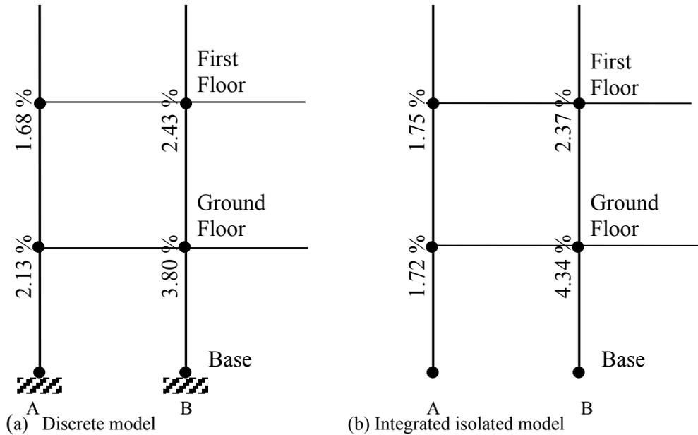
Figure 10 Discrete and integrated model column design rebar ratio
