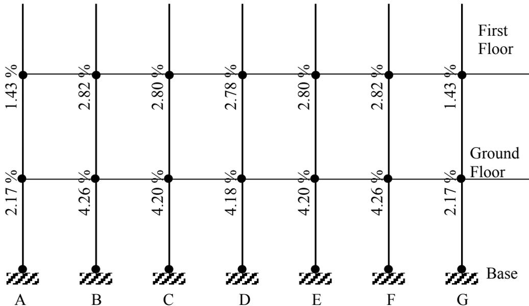
**Figure 4 Discrete model (columns design) rebar ratio**
