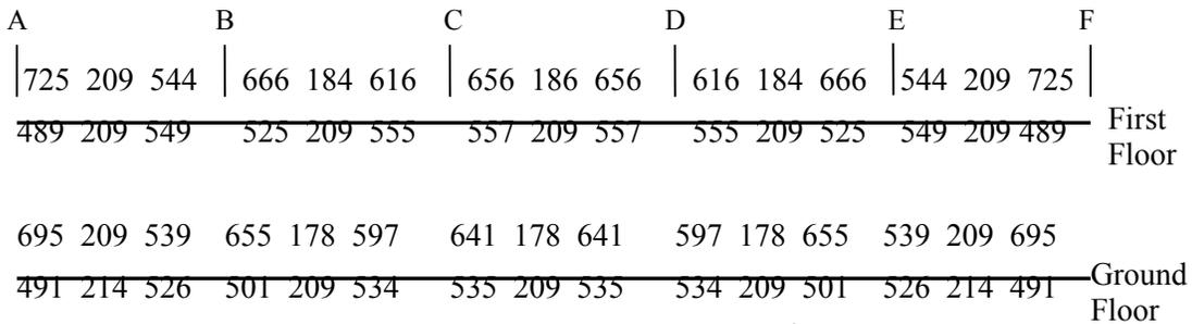
Figure 9. Integrated strip model (beam design steel area in mm<sup>2</sup>)
