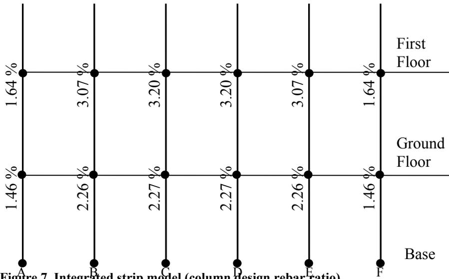
Figure 7. Integrated strip model (column design rebar ratio)
