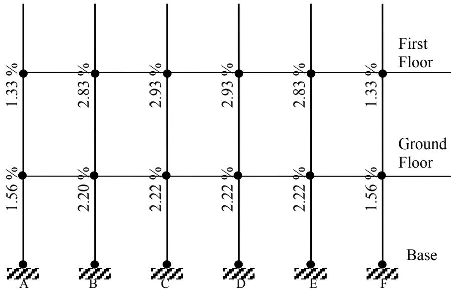
Figure 6. Discrete model (column design rebar ratio)
