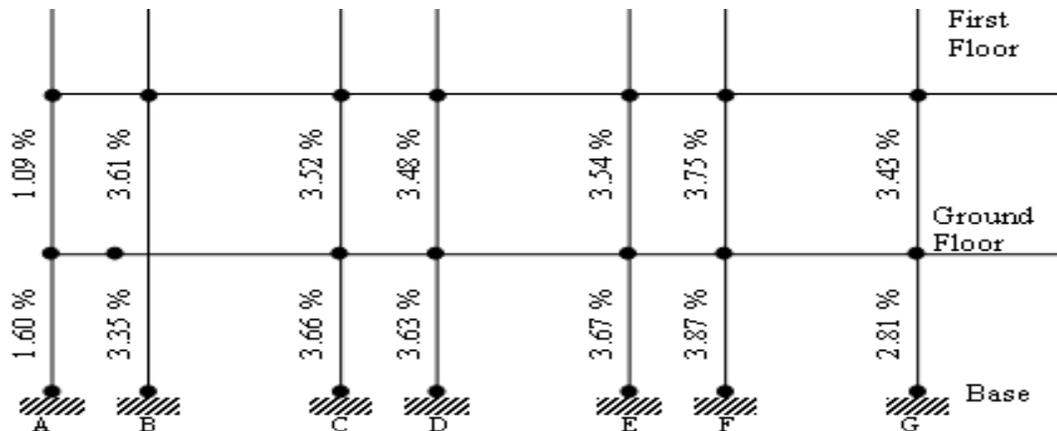
Figure 13 discrete models (column design rebar ratio)
