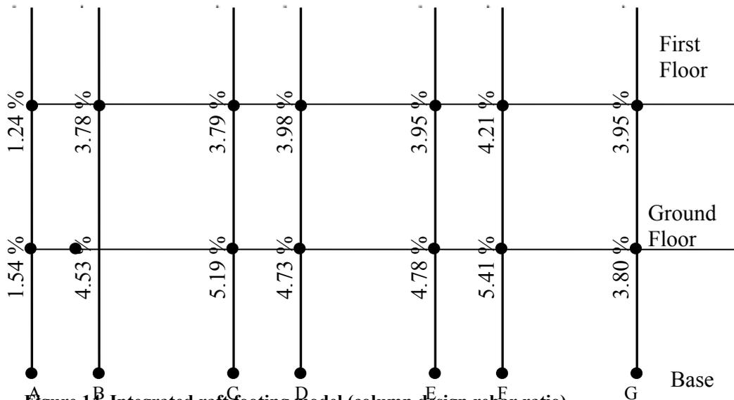
Figure 14. Integrated raft footing model (column design rebar ratio)
