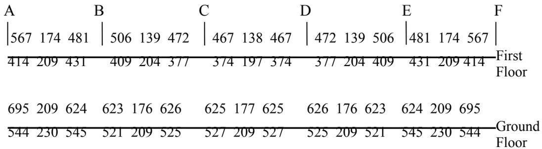
Figure 8. Discrete model (beam design steel area in mm<sup>2</sup>)
