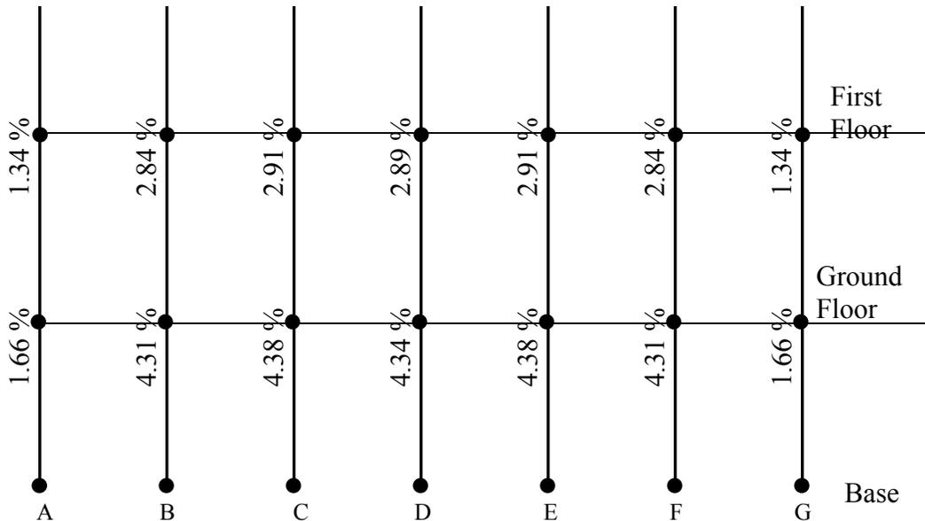
Figure 5 Integrated raft model (columns design) rebar ratio
