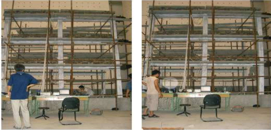
(b) 26kN Push and Pull at frame top Figure 4: Lateral loading cycles for PFT
